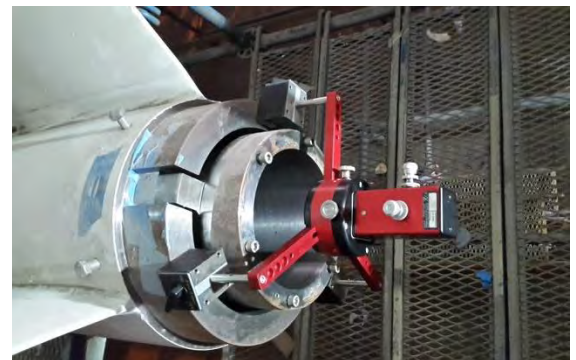
Laser transmitter on the aft V-bracket
