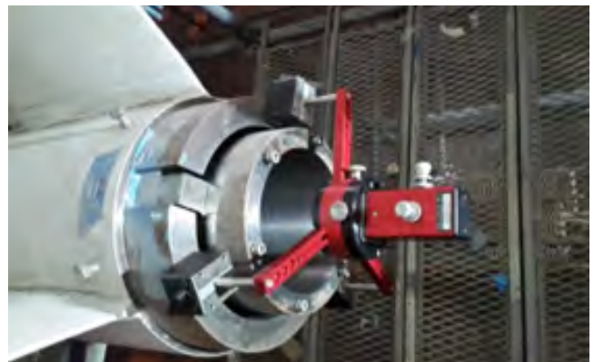
Laser transmitter on the aft V-bracket
