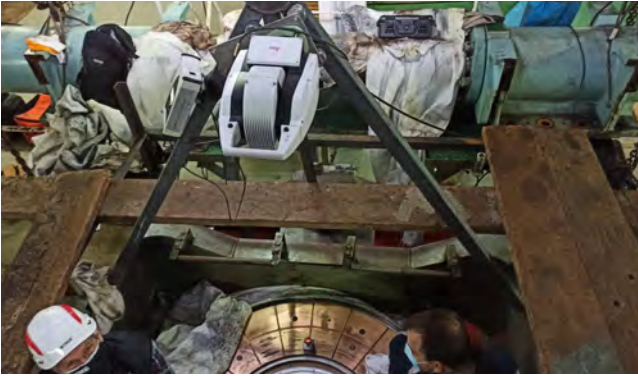
During measurements - Thrust Bearing Flatness Inspection
