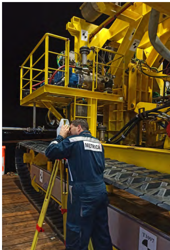
Laser scanner targets were surveyed during the measurement of control network
