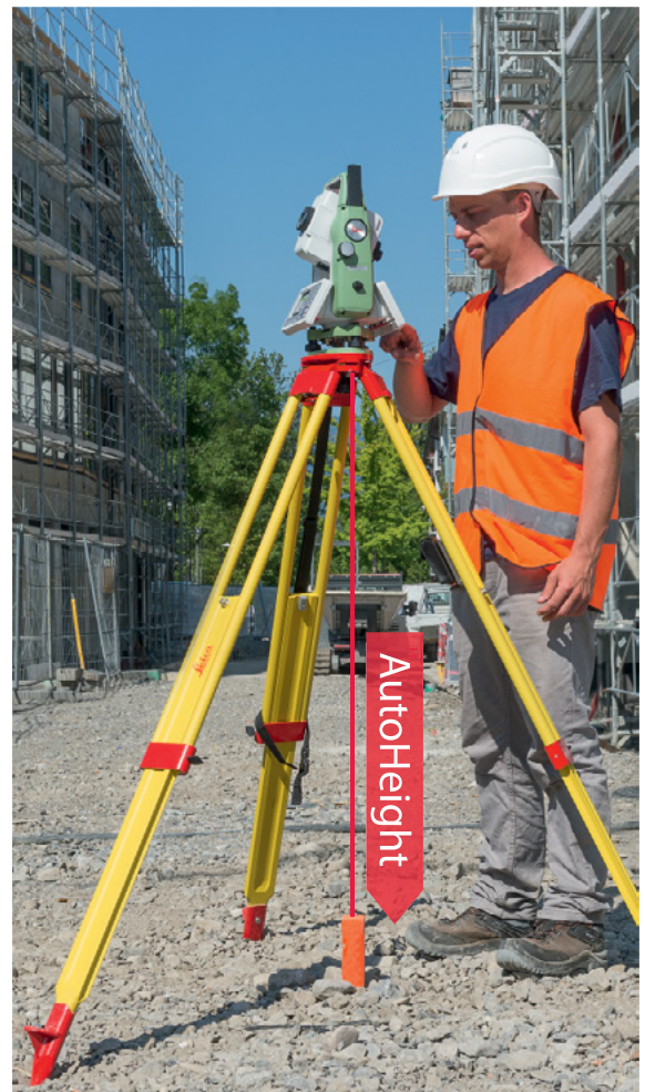
Figure 3 – Get your instrument height by simply pressing a button with the AutoHeight feature.
