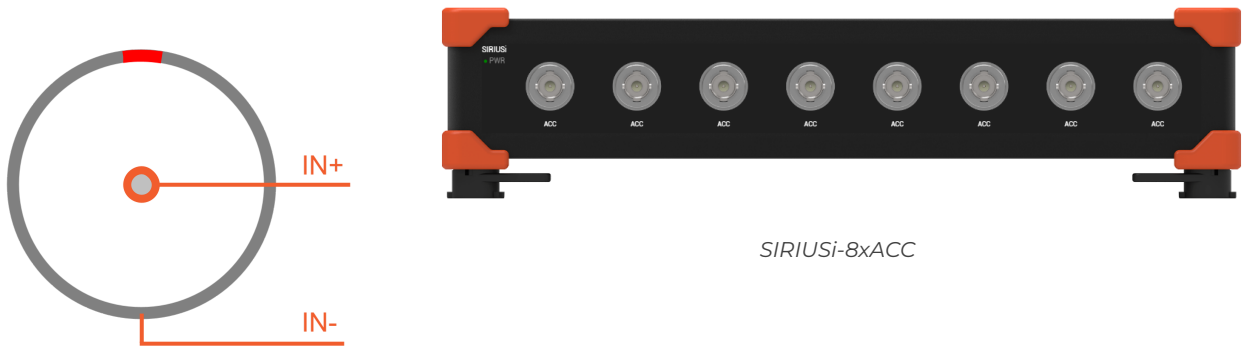
ACC connector: pin-out (BNC)
