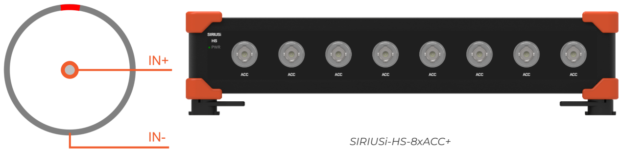
HS-ACC connector: pin-out (BNC)
